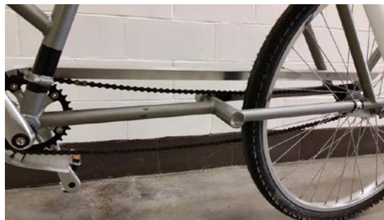
Figure 31. Shown above is the chain that does not have proper chain tension due to the dropouts not being long enough.
