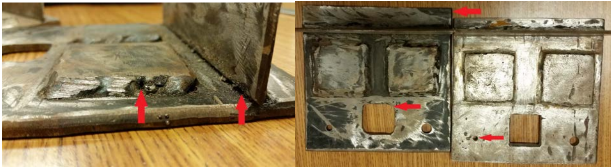
Figure 2. The welding quality in developing nations was of poor quality. The sample on the left shows very rough welding with burs, as well as connection completely missing the welding bead. On the right shows two samples made by different welders that were made from the same specs. The back section has different lengths, the left holes are of different sizes, and the square cutout has different corners.
