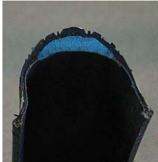
Figure 17. Tire filled with silicon. Silicon is colored in blue.
