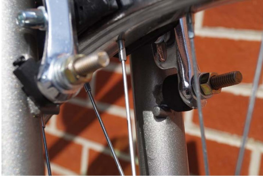
Figure 21. Front Brakes with modified mounting system.
