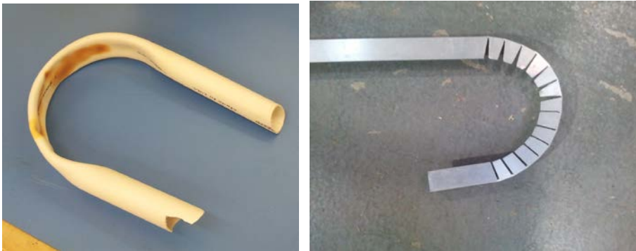
Figure 23. The initial chain guard design with heated and formed PVC tube on the left shows color changes where the heat burnt the plastic, causing brittleness. The final chain guard on the right, was made from aluminum, and formed around a pipe, after grooves were cut.
