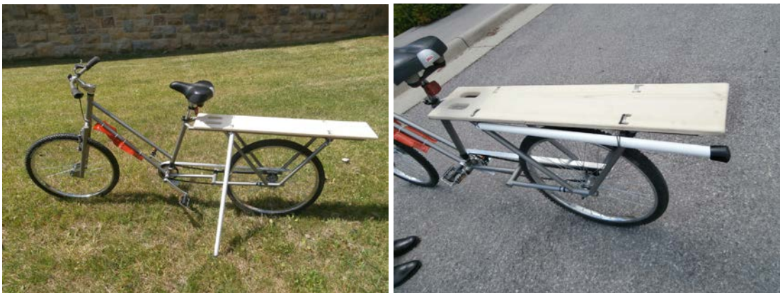
Figure 22. PVC kickstand design on the left, holding up the load at the rack to greatly reduce the moment compared with typical kickstand placement. The wire cradle attached to the frame can be seen on the right storing the kickstand for transport.
